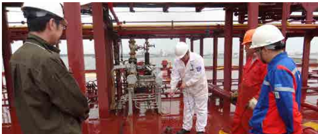
Crude oil being sampled by a third-party commodity inspector
