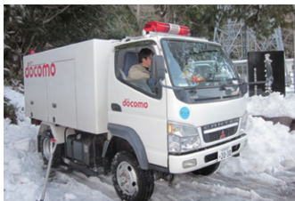
Power supply vehicle dispatched for the prompt restoration of communications services
