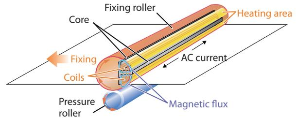
An electromagnetic induction heater induces an eddy current when magnetic flux passes through metal coils, causing the fixing roller to emit heat. In this way, overall heat efficiency is improved and energy consumption is reduced.
