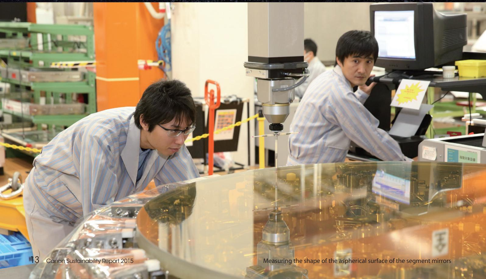
Measuring the shape of the aspherical surface of the segment mirrors
