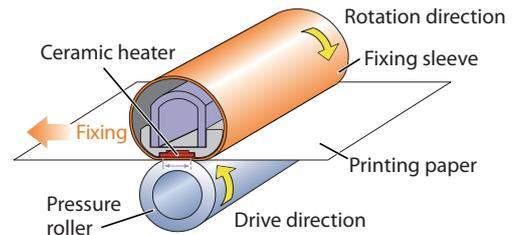
The use of a ceramic heater that heats up quickly and a fixing sleeve that transfers heat efficiently allows for localized heating of the fixing point and instantaneous heat transfer. No excess electricity is consumed in standby mode, enabling a shorter warm-up period.
