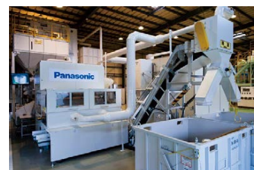
PETEC resin selection machine using near-infrared identification technology
