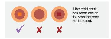
The HEATmarker® is a miniaturized, self-adhesive temperature indicator affixed to vaccine packaging at the time of manufacture. It provides an easy tool to identify whether a vaccine has been exposed to heat damage. Without such a system, consumers have no means of ascertaining whether the vaccine they will receive has been properly stored and handled before it is administered.
