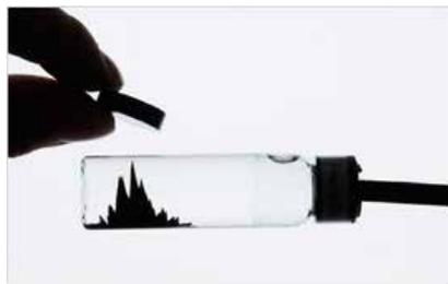
Magnetic fluid reacting to the magnetic force
