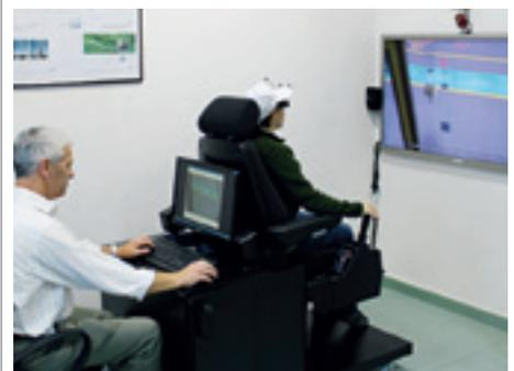
*Our Research & Development teams have developed a special simulator that uses the latest virtual reality techniques to help train crane operators. Replicating the actual experience of working the crane through state-of-the-art graphics, sound systems, LCD projectors, and movement sensors help to improve the skills of inexperienced workers, and increases safety throughout our operations.*
