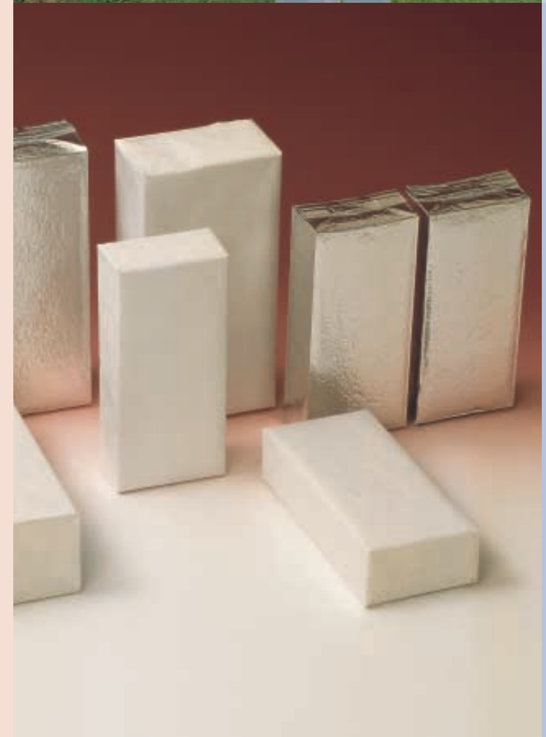
Product protection comprises the core competence in packaging technology. Foodstuffs lose quality through contact with oxygen. Inert-gas packaging or evacuation facilitates the reduction of residual oxygen to less than 2%. Packaged coffee is but one example.
